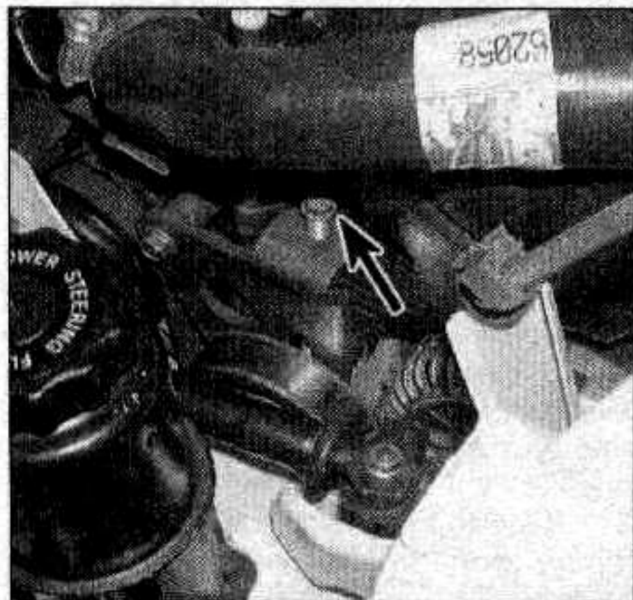
12.5a On V6 models, loosen the tensioner locknut (in the center of the adjuster pulley) and turn the adjuster bolt (arrow) to adjust the alternator and air conditioning compressor belt tension
