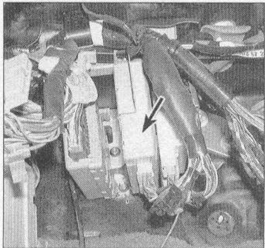
2.2a Location of the ABS control module (arrow) under the left side of the instrument panel
