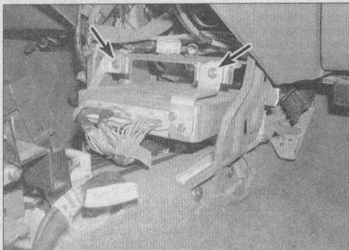
3.3 Disconnect the PCM electrical connectors then remove the mounting bolts (arrows)
