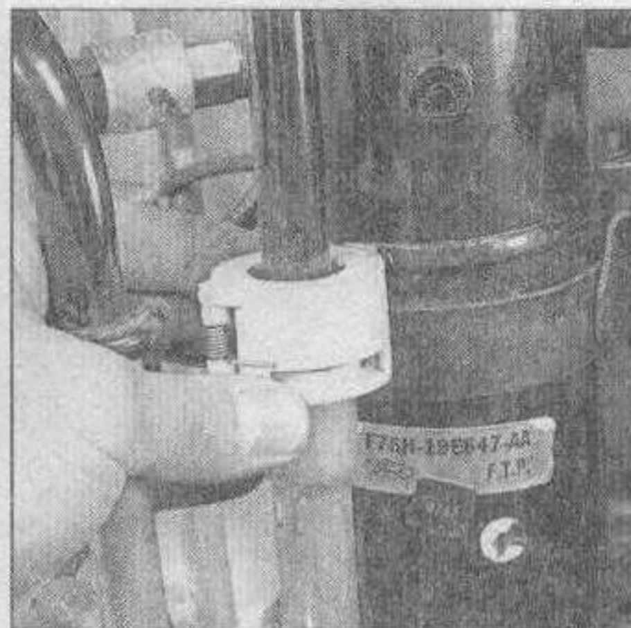
16.3b Where spring-lock couplings are used in refrigerant lines, use a spring-lock coupling tool - clamp the tool over the connection while pushing the two lines toward each other, then pull outward to release (typical example shown)
