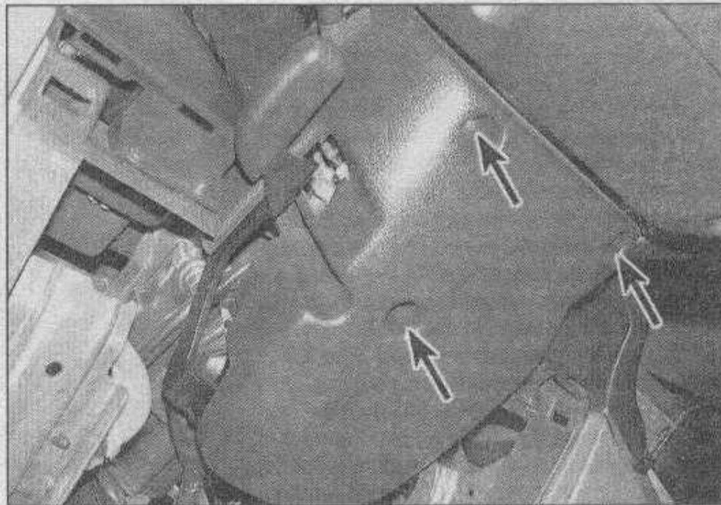
29.2 Remove the screws (arrows) at the lower column cover, then remove the upper and lower covers
