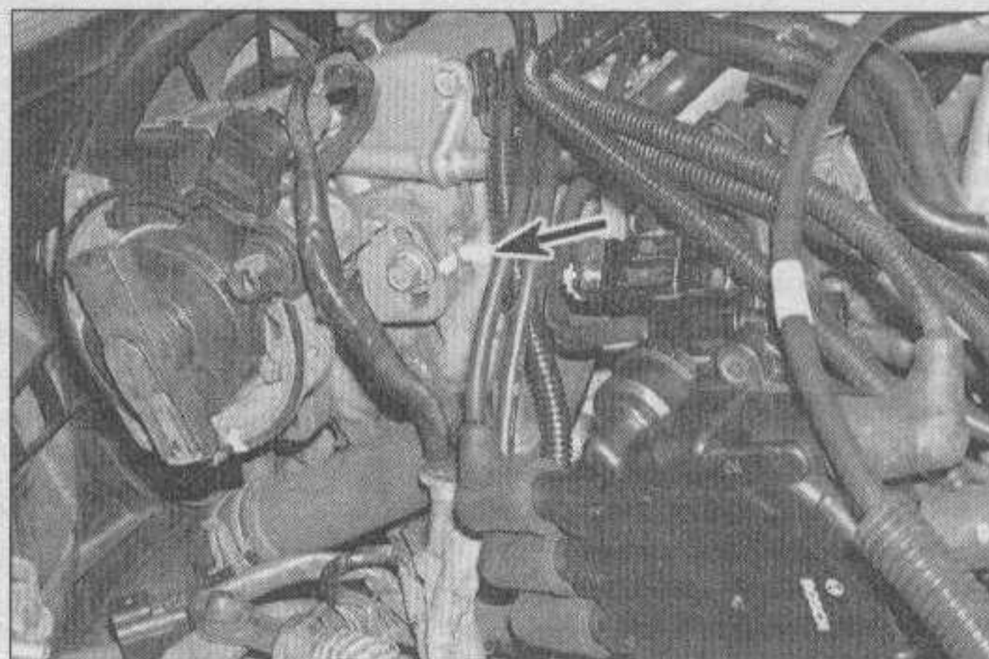
9.5b Mark the position of the distributor body in relation to the cylinder head (arrows) using white paint
