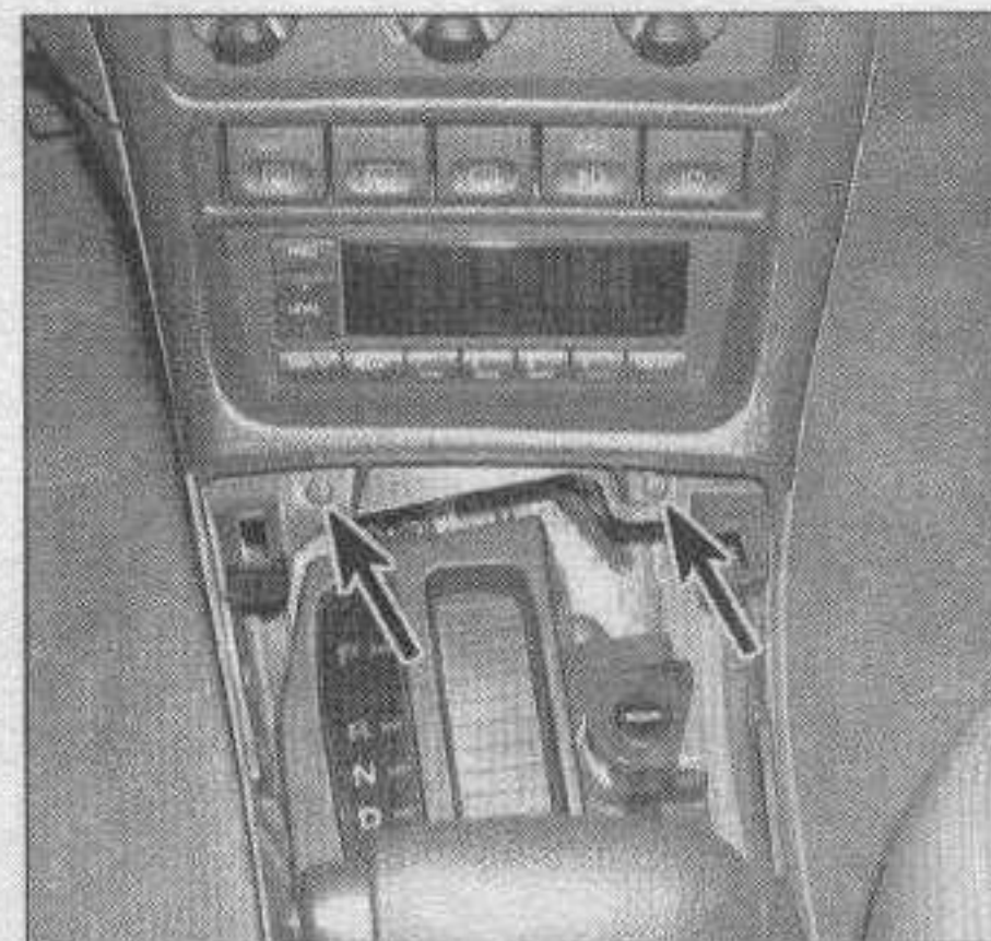
27.7a Remove the screws (arrows) at the front edge of the console
