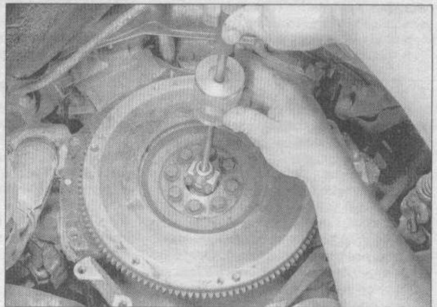
6.13 A small slide hammer is handy for removing a pilot bearing
