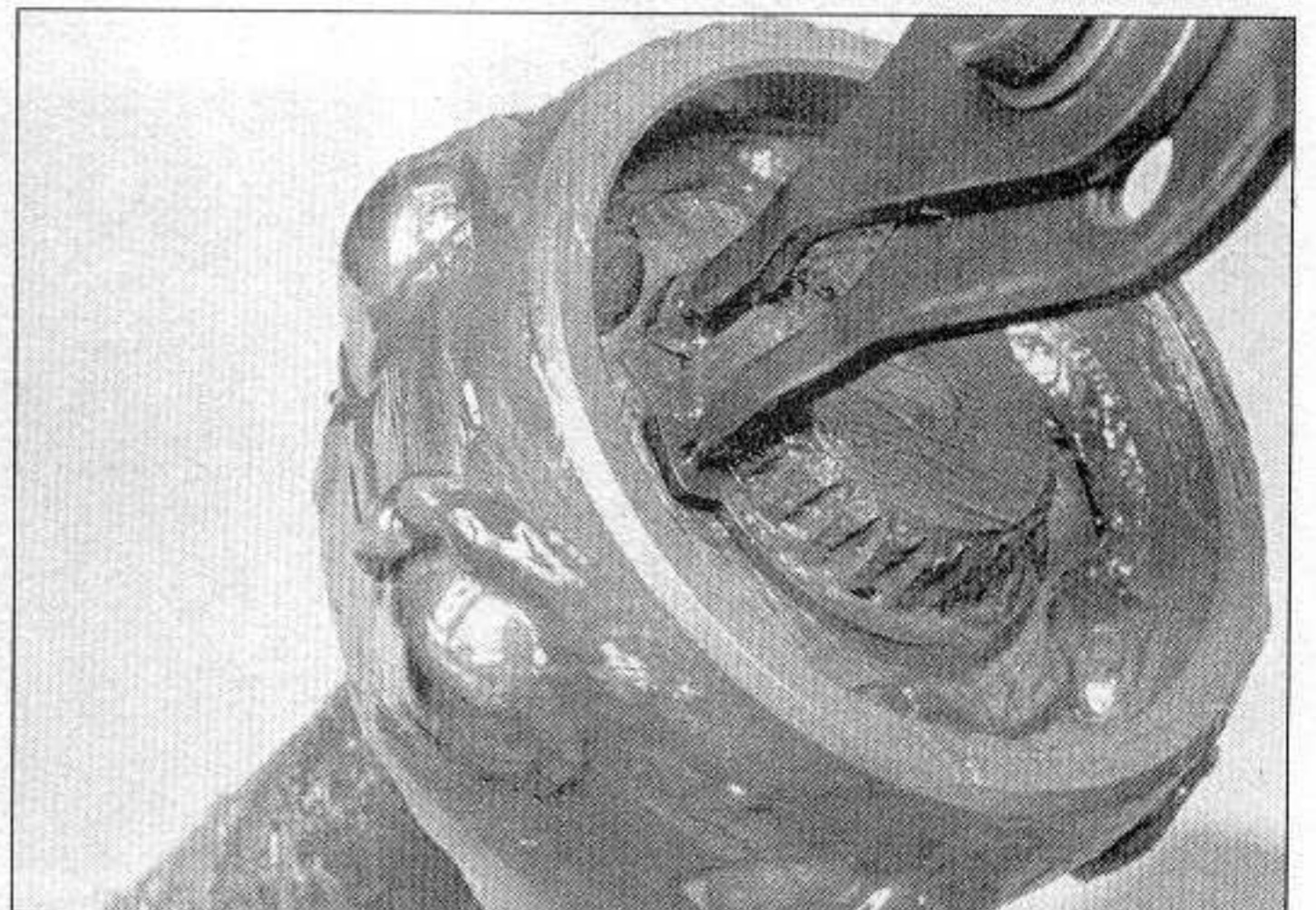
13.20 Remove the snap-ring from the end of the axleshaft
