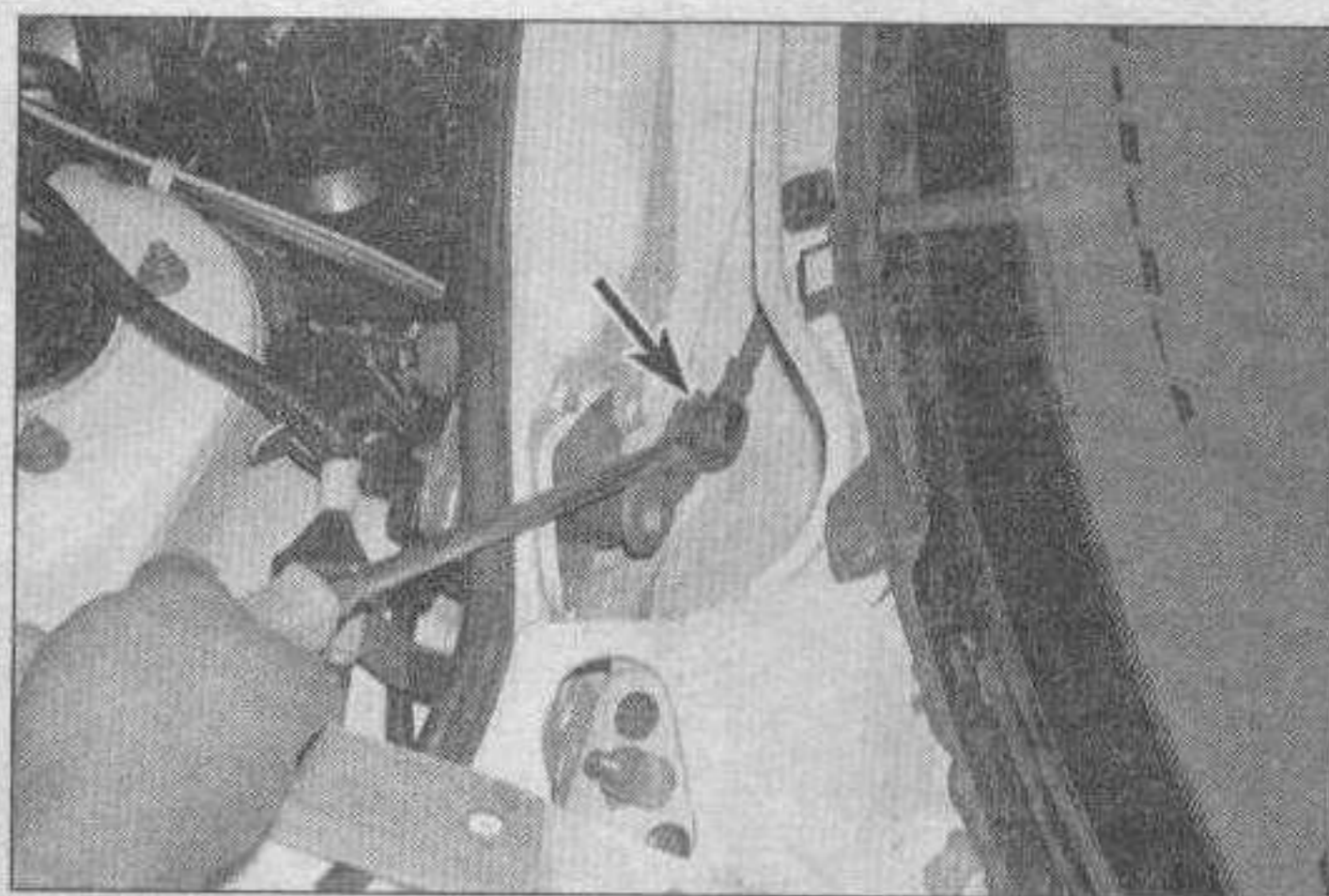
19.9 Pry the linkage arm off the wiper pin (arrow) with a large screwdriver
