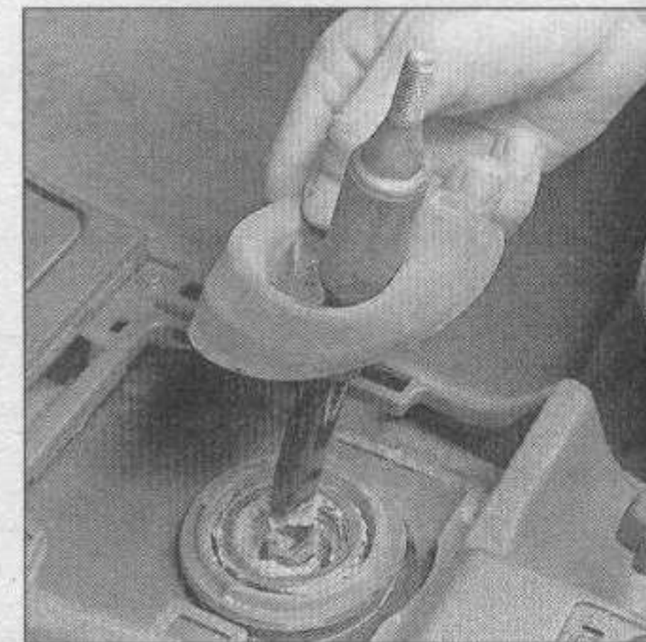
2.4 Remove the boot from the lower end of the shift lever assembly
