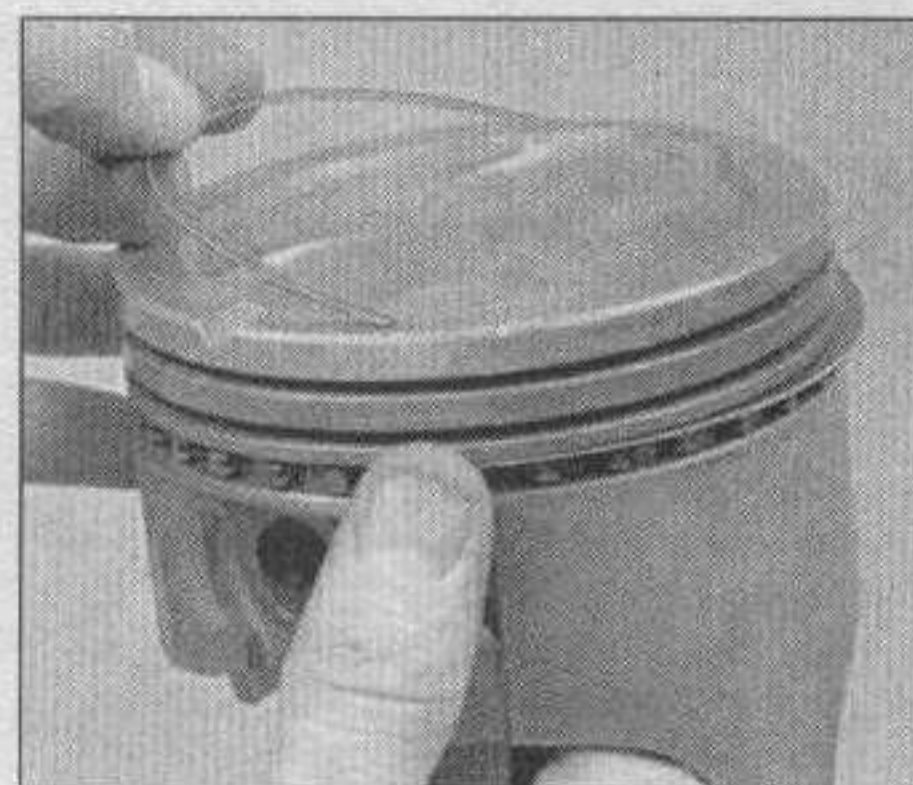
23.9b DO NOT use a piston ring installation tool when installing the oil ring side rails
