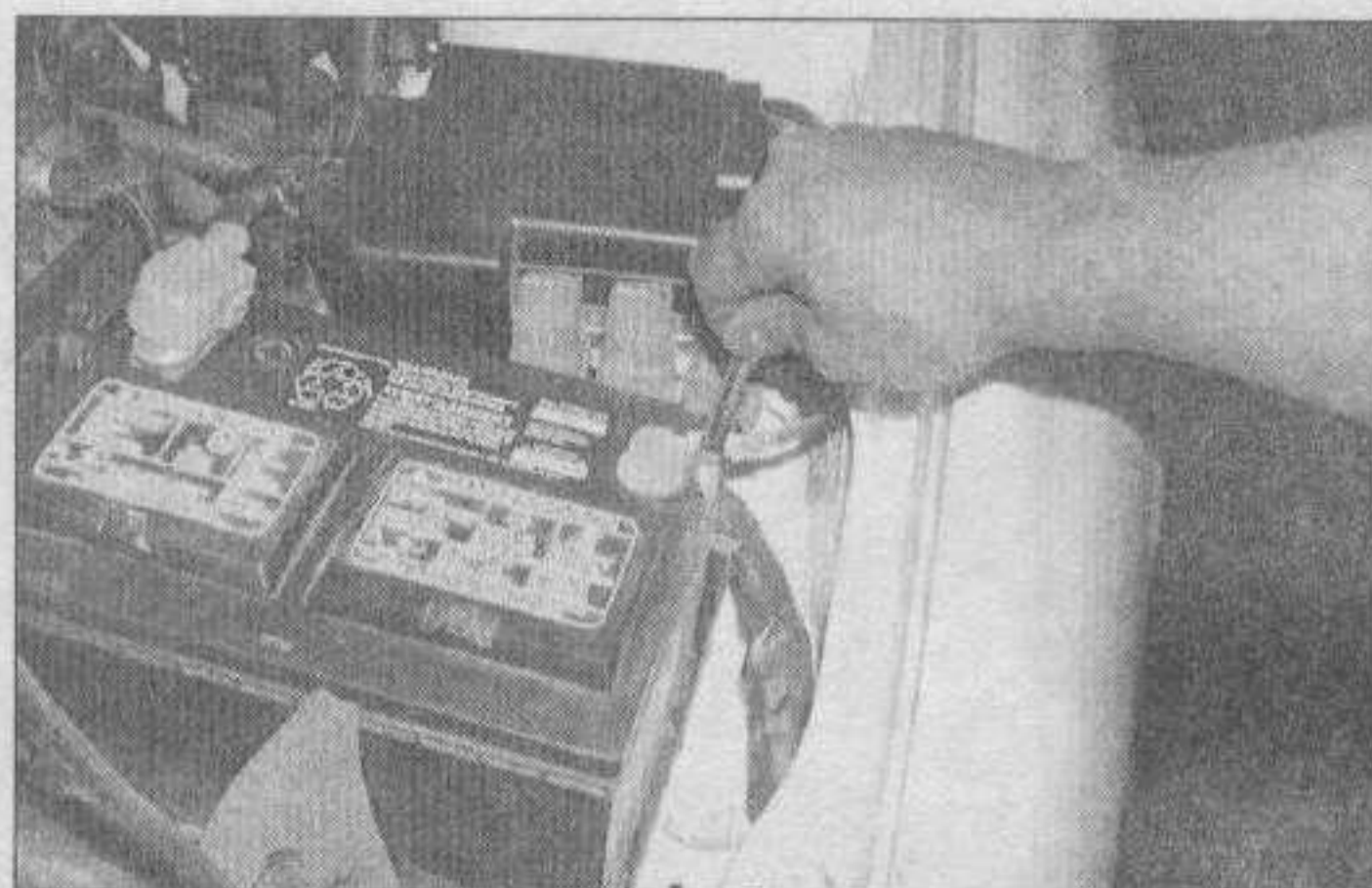
4.4a Removing the cable from a battery post with a wrench - always remove the negative cable first and hook it up last!
