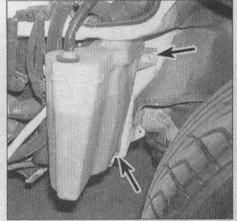
5.1b . . . and the two bolts (arrows) in the fenderwell (fender removed for clarity)
