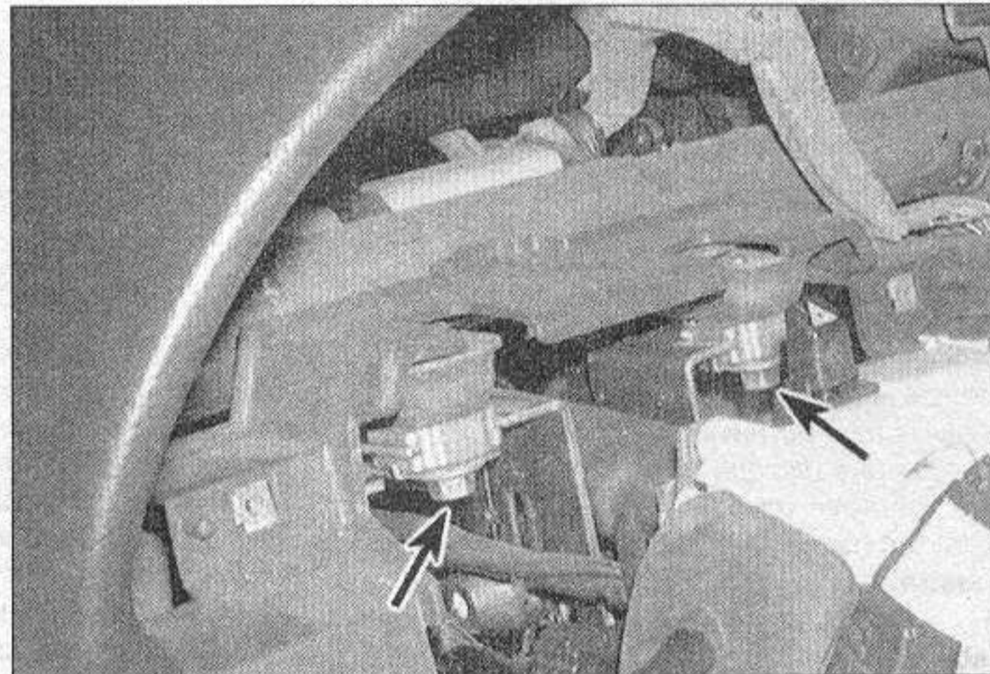
15.10 Remove the steering column mounting bolts (arrows)
