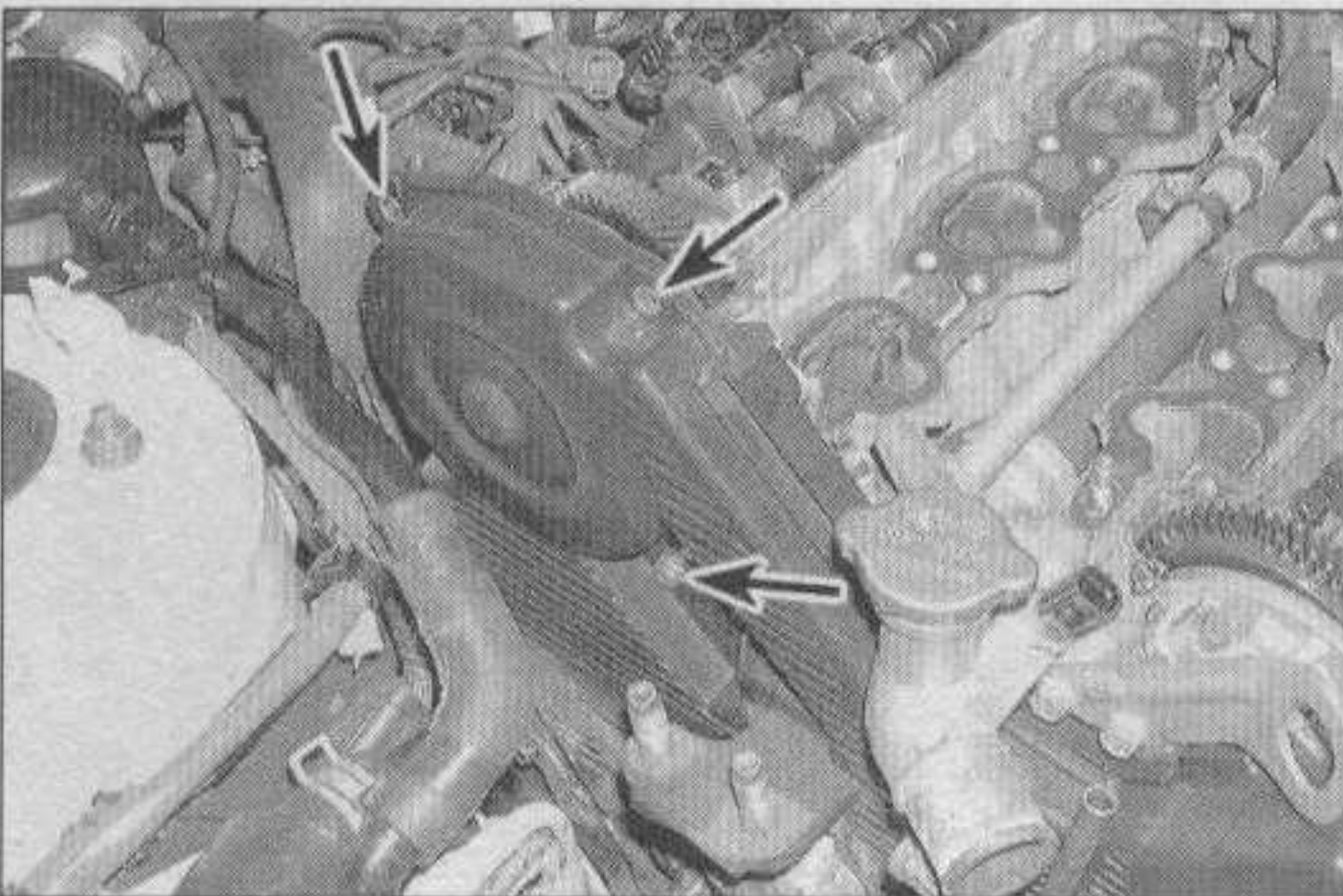
6.14b Remove the three upper bolts (arrows) and the timing belt cover
