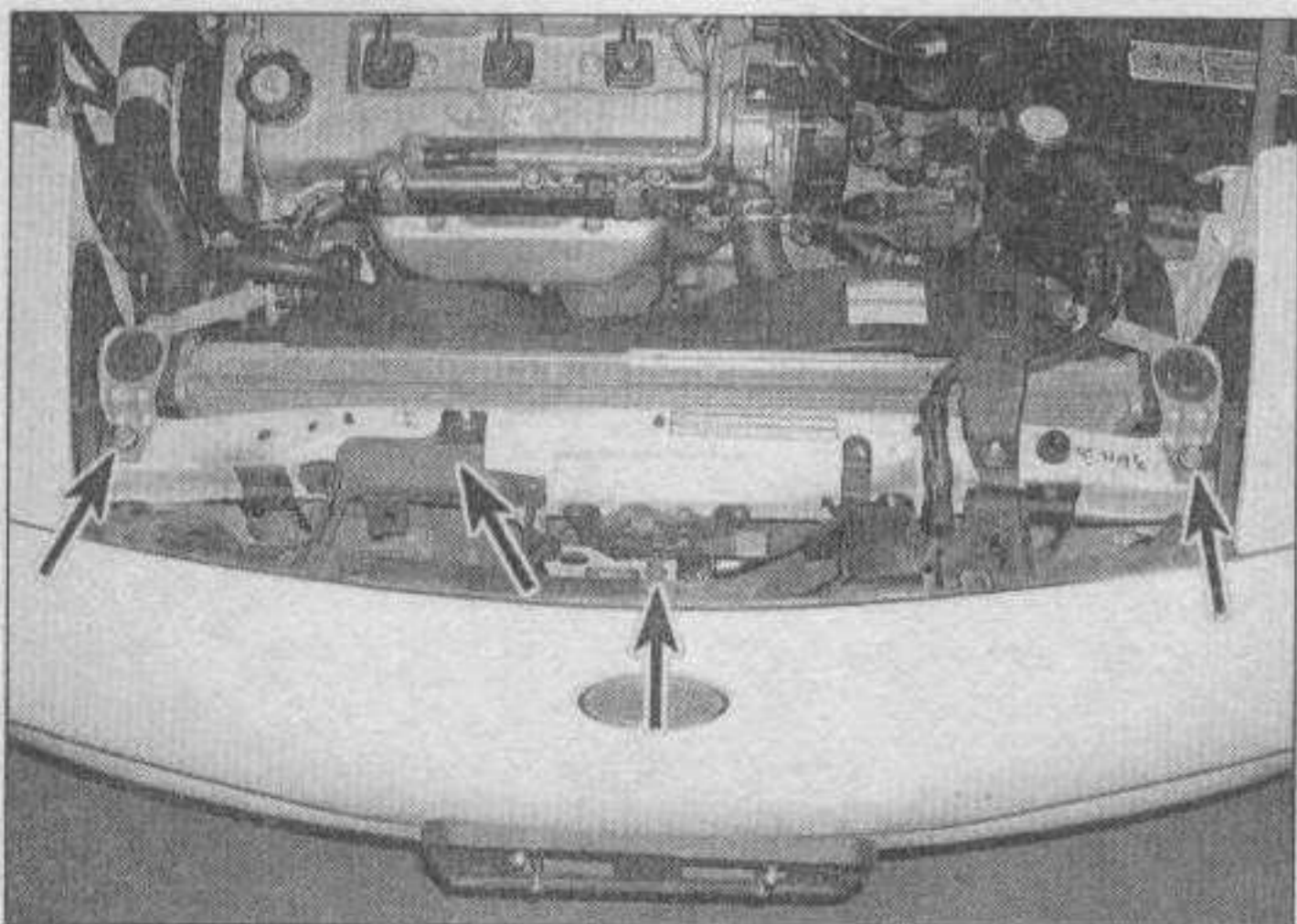
12.3a Remove the air deflector, radiator support and bumper cover support bracket screws (arrows)
