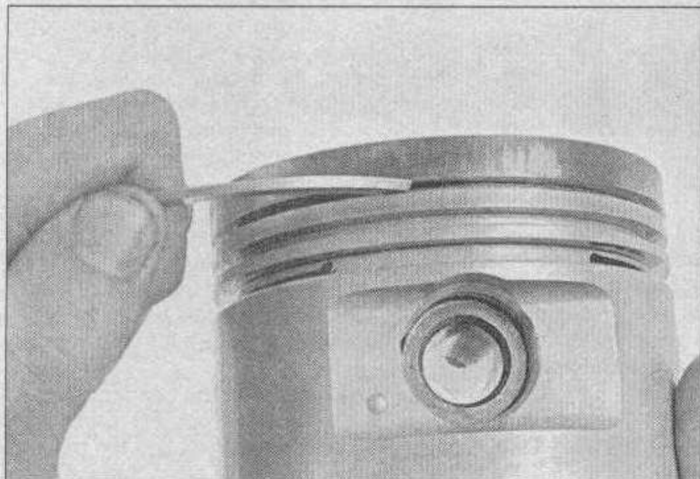
18.4b . . . or a section of a broken ring
