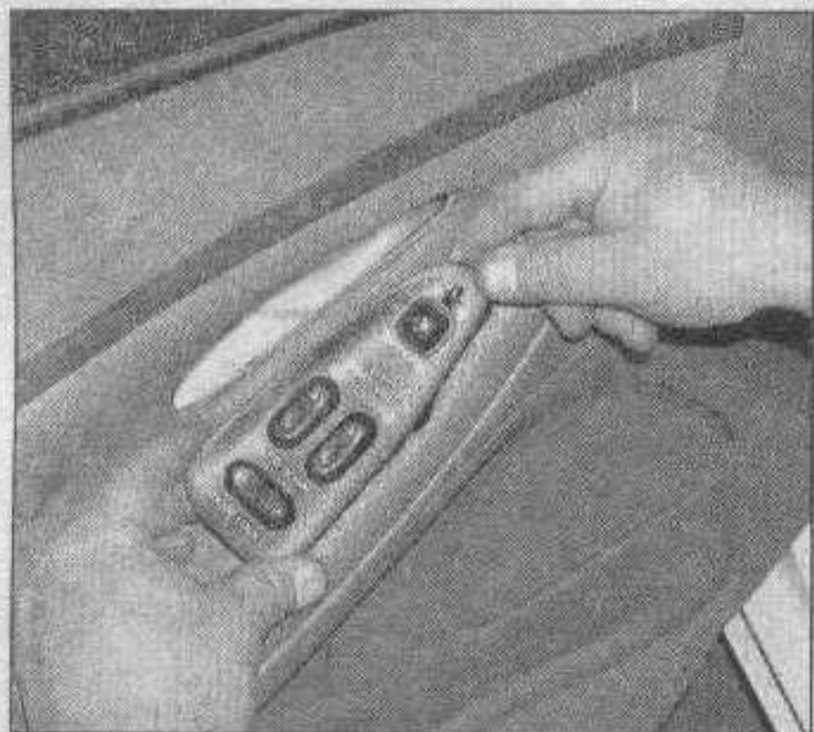
15.4 Carefully lift the switch assembly out of the trim panel and rotate it out far enough to disconnect the electrical connectors
