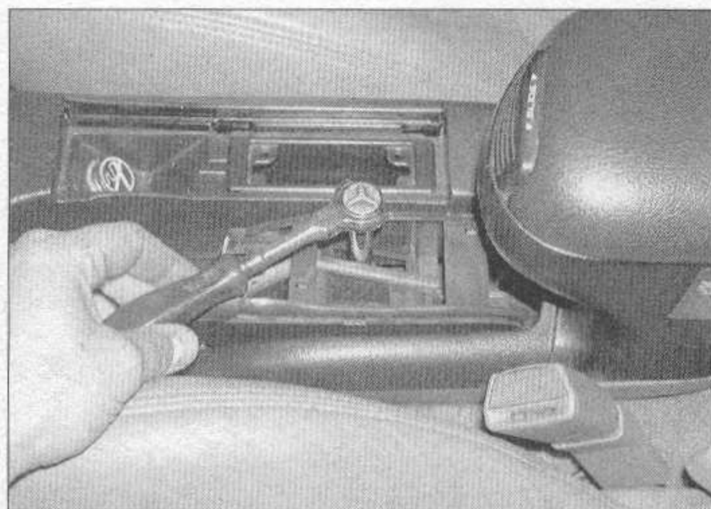
13.3 Location of the parking brake cable adjusting nut on a Ford Probe equipped with an automatic transaxle
