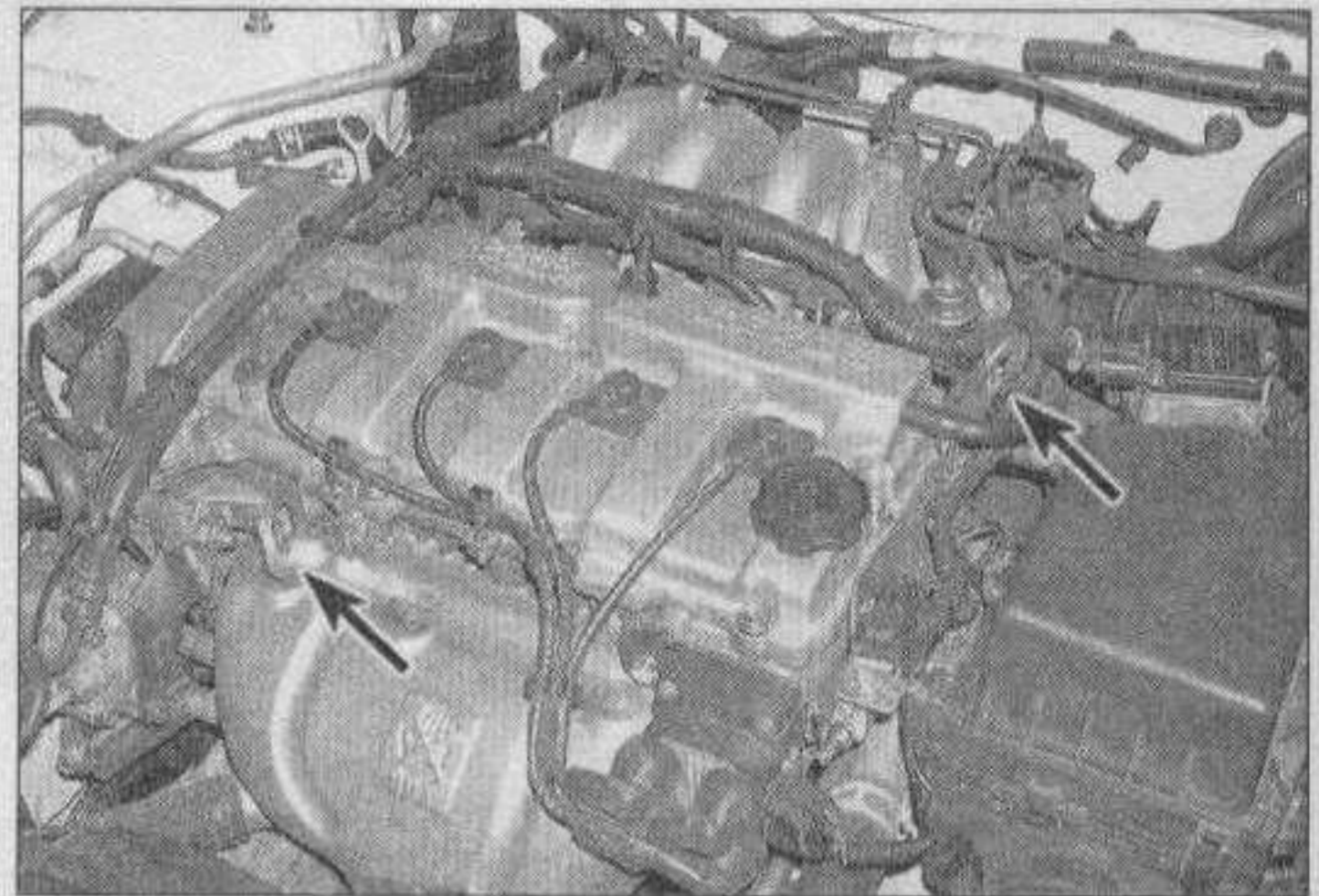
7.20 Attach a sling or chain securely-fastened with bolts/nuts to the two lifting eyes (arrows) - four-cylinder shown, V6 similar
