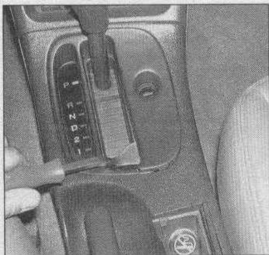
27.2 With a tool like this one or a taped screwdriver, pry out the shift bezel
