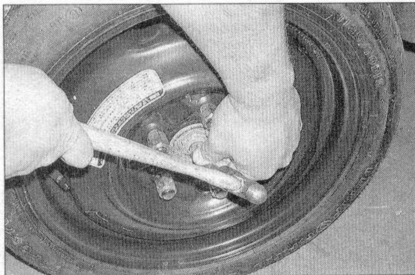
4.1 Unstake the driveaxle/hub nut using a chisel and hammer
