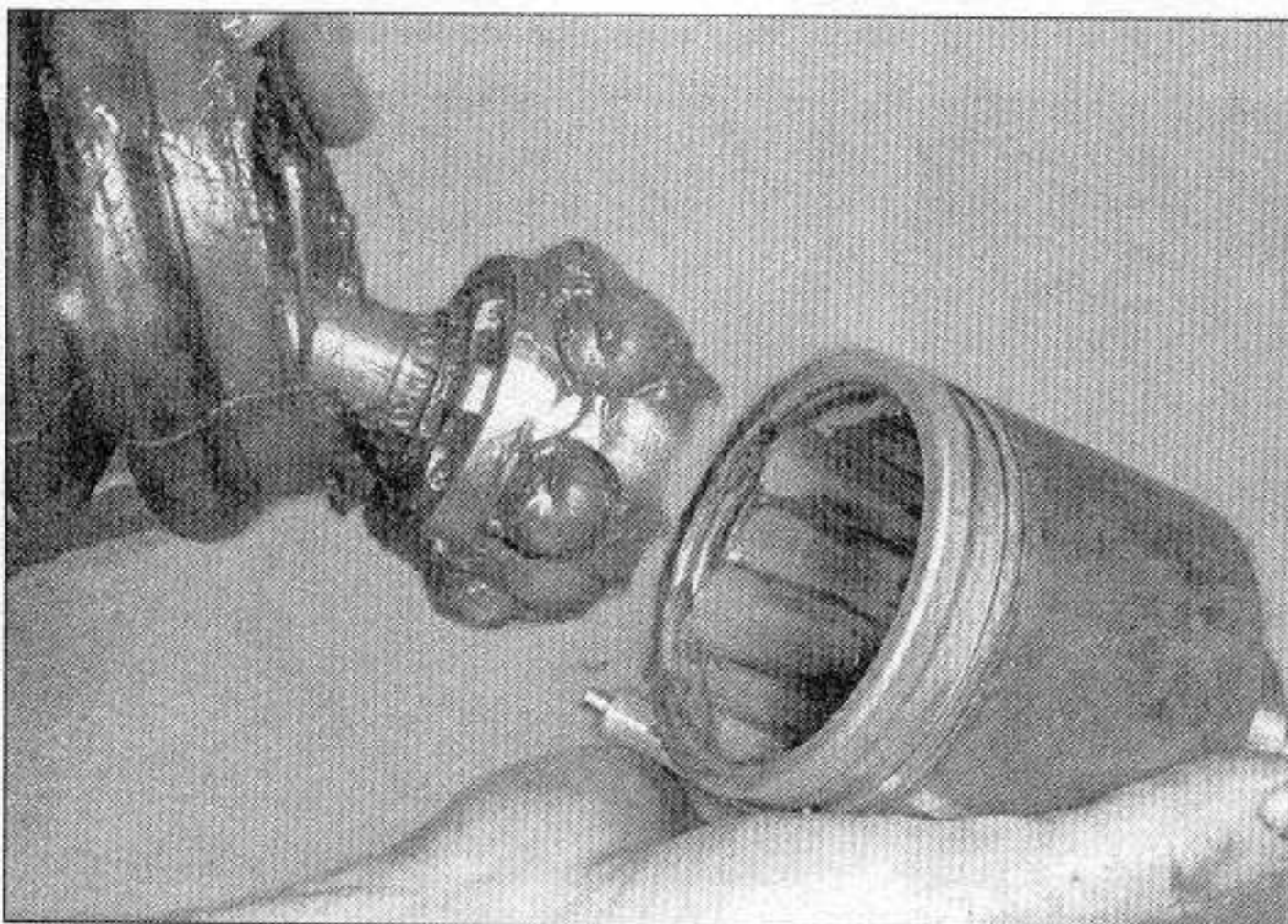
13.19 With the retainer removed, the CV joint housing can be pulled off the ball-and-cage bearing assembly
