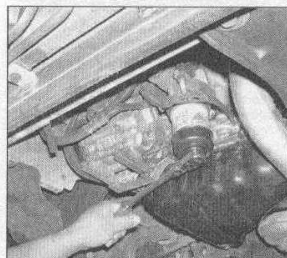
8.12 The oil filter is usually on very tight and will require a special wrench for removal - DO NOT use the wrench to tighten the new filter
