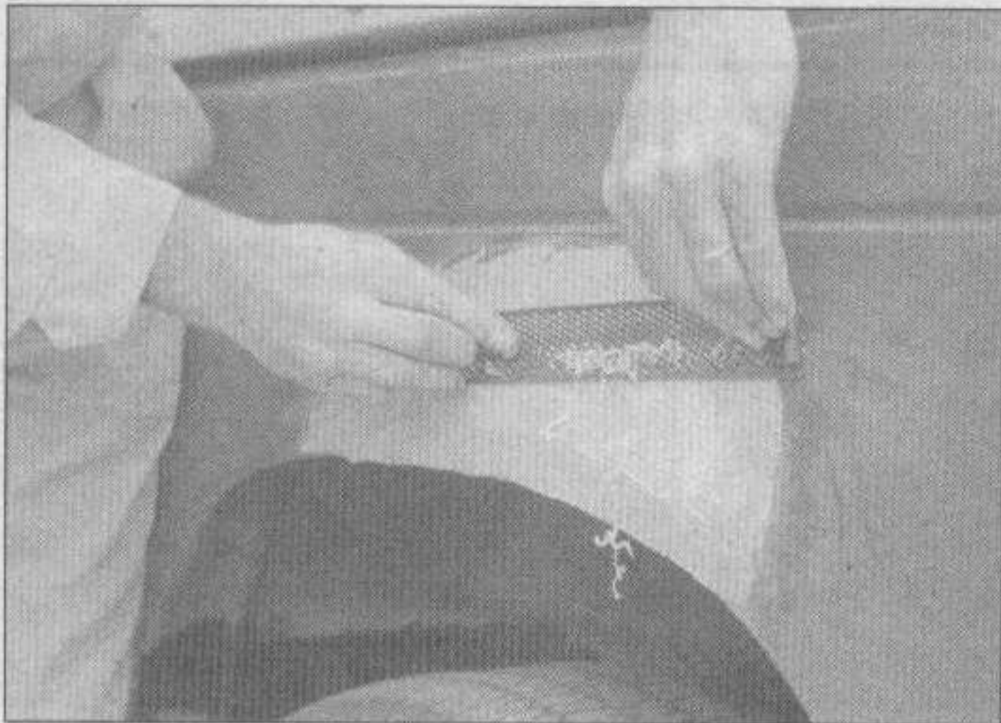
7 Let the filler harden until you can just dent it with your fingernail. Use a body file or Surform tool (shown here) to rough-shape the filler
