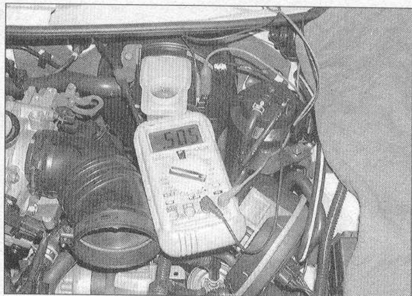
15.2 Use an ohmmeter to check the brake fluid level switch - with the float in the UP position, there should be no continuity
