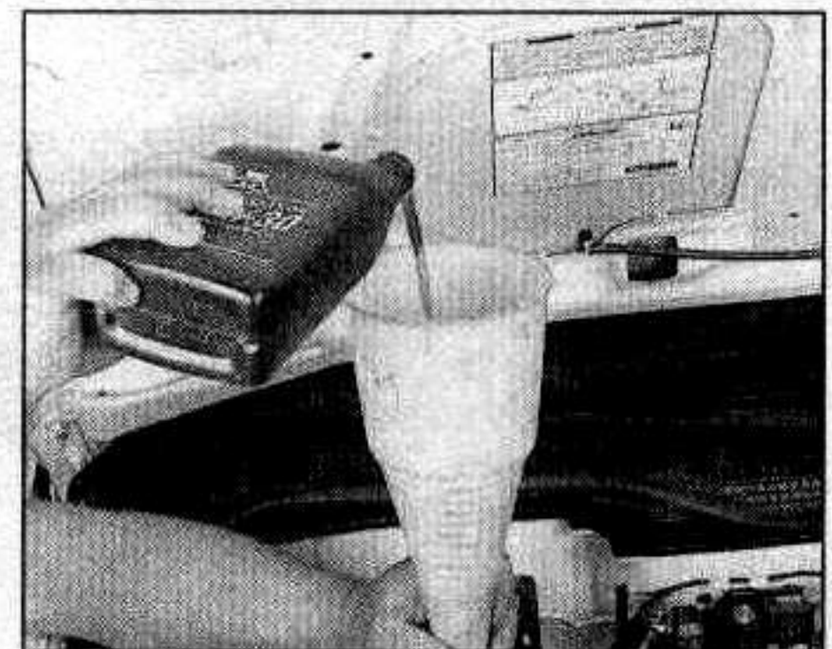
17.2b . . . so you can easily add lubricant to the transaxle from above
