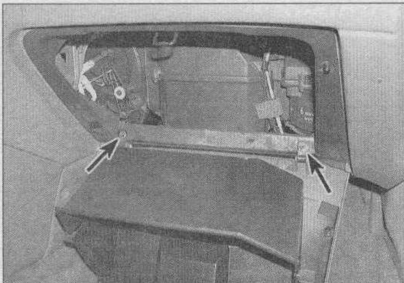
28.15 Remove the glove box hinge screws (arrows)
