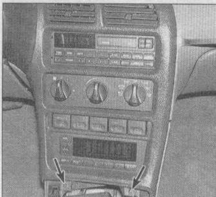
28.12 Remove the screws (arrows) and pry the center instrument panel free of the instrument panel
