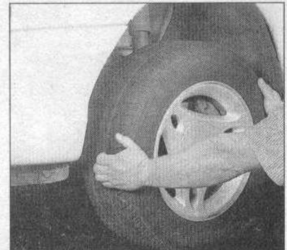
26.11 With the steering wheel in the lock position and the vehicle raised, grasp the front tire as shown and try to move it back-and-forth - if any play is noted, check the steering gear mounts and tie-rod ends for looseness
