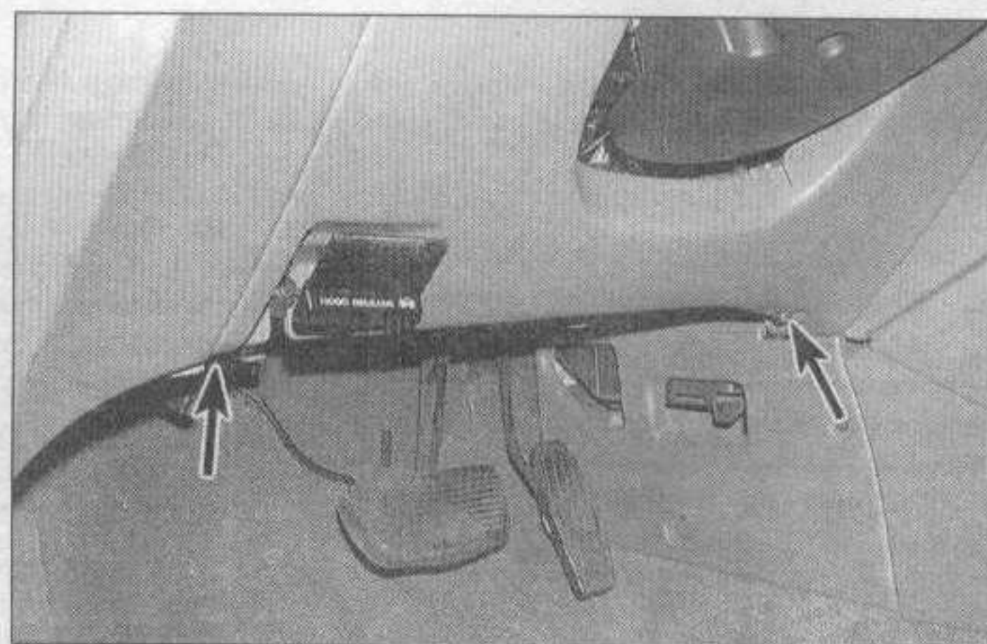
28.9 Remove the screws (arrows) and detach the knee bolster
