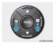
The fan speed can be set to the desired speed by operating the fan speed control switches.
