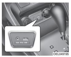
If your vehicle has an aux and/or USB(universal serial bus) port, you can use an aux port to connect audio devices and the USB port to plug in a USB device.
