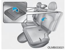
Pull up the seatback lever, then fold the seat toward the front of the vehicle.
