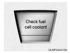
This warning message illuminates if the coolant level in the fuel cell stack coolant reservoir is low. To refill the coolant, consult an authorized HYUNDAI Tucson Fuel Cell dealer.
