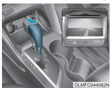
The Rear View Camera will activate when the power cell module is running and the shift lever is in the R (Reverse) position.
