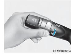
Fog lights are used to provide improved visibility when conditions are poor due to fog, rain, snow, etc.
