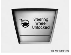
This warning message illuminates if the steering wheel does not lock when the POWER button changes to the OFF position.
