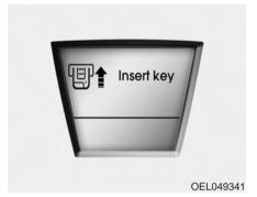
This warning message illuminates if you press the POWER button while the warning message "Key is not detected" is being displayed on the LCD display. Also, the immobiliser indicator and the smart key holder light blinks for a while.
