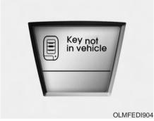
This warning message illuminates if the smart key is not in the vehicle when you press the POWER button.
