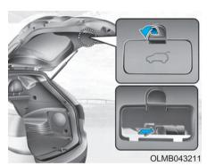
Your vehicle is equipped with an Emergency Tailgate Safety Release lever located inside on the bottom of the tailgate. When someone is inadvertently locked in the luggage compartment, the tailgate can be opened by moving the lever in the direction of the arrow and pushing the tailgate open.
