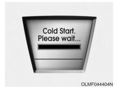
When attempting to start the vehicle in cold weather (below freezing conditions), the power cell module may need more time than normal to achieve the READY state.
