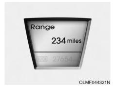
This mode indicates the estimated distance to empty based on the current fuel in the fuel tank and the amount of fuel delivered to the power cell module. When the remaining distance is below 30 miles (50 km), "----" will be displayed and the distance to empty indicator will blink.
