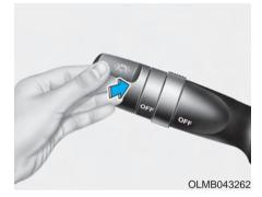
To turn on the high beam headlights, push the lever away from you. Pull it back for low beams.
