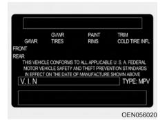
The certification label is located on the driver's door sill at the center pillar and shows the maximum allowable weight of the fully loaded vehicle. This is called the GVWR (Gross Vehicle Weight Rating). The GVWR includes the weight of the vehicle, all occupants, fuel and cargo.
