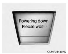
. If you turn off the vehicle at the low temperature, a blower will work to terminate the fuel cell electric system operation.
