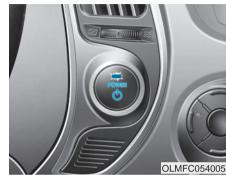
Whenever the front door is opened, the POWER button will illuminate and will go off 30 seconds after the door is closed.
