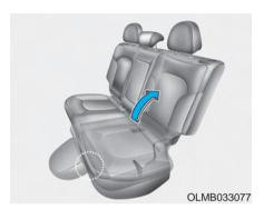
7. To use the rear seat, lift and push the seatback backward. Push the seatback firmly until it clicks into place. Make sure the seatback is locked in place.
