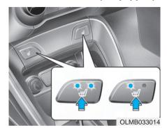
While the power cell module is running, push either of the switches to warm the driver's seat or front passenger's seat.
