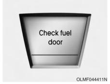
When the fuel filler door is not closed securely, this warning message illuminates. The vehicle cannot be driven if the fuel filler door is open. Make sure the fuel filler door is closed before starting the vehicle.
