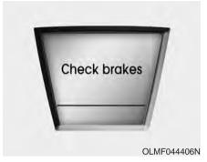
This warning message illuminates if the brake system needs to be checked. Have the vehicle inspected by an authorized HYUNDAI Tucson Fuel Cell dealer.
