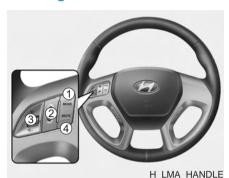
The steering wheel may incorporate audio control buttons. These buttons are installed to promote safe driving.
