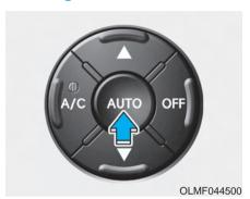
When using the AUTO climate control mode, the fan speeds, mode selection, air intake control, and the air conditioning will be automatically controlled according to the desired temperature setting.
