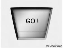
This message illuminates if you have started the vehicle properly and there is no malfunction (Also, the READY indicator light comes on).
