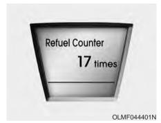
A refueling counter is set up in the instrument cluster to monitor the number of times the hydrogen storage tank is pressurized. After refueling, the Refuel Counter will indicate the number of times the vehicle has been refueled.
