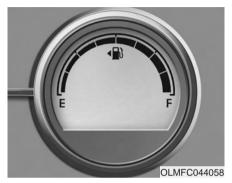
This gauge indicates the approximate amount of fuel remaining in the fuel tank (The fuel tank capacity is given in chapter 8). The fuel gauge is supplemented by a low fuel warning light which will illuminate when the fuel tank is nearly empty.
