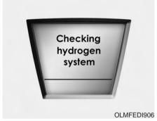
This warning message illuminates for about 10 seconds and then disappears if a malfunction is detected on the sensor for the fuel filler door while refuelling (While this message is being displayed on the LCD display, you can not start the vehicle). If you have experienced this warning message, have the vehicle inspected by an authorized HYUNDAI Tucson Fuel Cell dealer.
