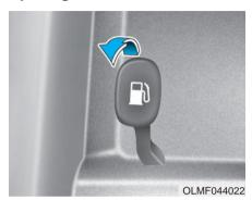
The fuel filler door opener lever is located on the floor on the left side of the driver's seat. The fuel filler door must be opened from inside the vehicle. To open the fuel filler door:
