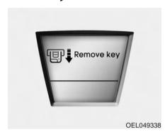
This warning message illuminates and the smart key holder light blinks if you turn off the vehicle with the smart key still in the smart key holder.
