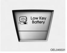
This warning message illuminates when the battery of the smart key is low. The warning message illuminates after the vehicle is shut down (POWER button changes to the OFF position).
