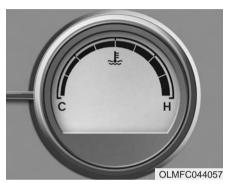
This gauge shows the temperature of the fuel cell stack coolant when the POWER button is ON.
