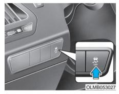
The Electronic Stability Control (ESC) system helps to stabilize the vehicle during cornering maneuvers. ESC checks where you are steering and where the vehicle is actually going. ESC applies braking pressure to any one of the vehicle's brakes and intervenes in the power cell module management system to assist the driver with keeping the vehicle on the intended path. It is not a substitute for safe driving practices. Always adjust your speed and driving to the road conditions.
