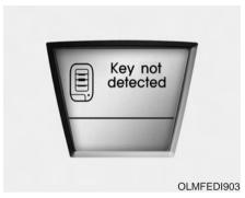
This warning message illuminates if the smart key is not detected when you press the POWER button.
