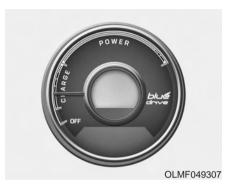
This gauge indicates the power consumption amount of the traction motor or charging amount of the high voltage battery.
