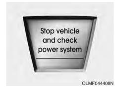
· This warning message illuminates if a severe malfunction is detected on your vehicle. At that time, park the vehicle cautiously as soon as possible, turn off the vehicle, and then try to start the vehicle again. After that, if this warning message remains, have the vehicle inspected by an authorized HYUNDAI Tucson Fuel Cell dealer
