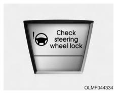
This warning message illuminates if the steering wheel does not lock normally when the POWER button changes to the OFF position.
