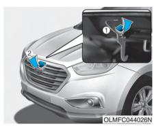
3. Raise the hood slightly, pull the secondary latch (1) inside of the hood center until it releases the hood and lift the hood (2).
