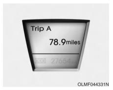
This mode indicates the distance of individual trips selected since the last tripmeter reset.
