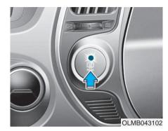
The defroster heats the window to help remove frost, fog and thin ice from the rear window, while the vehicle is in the "READY" state.
