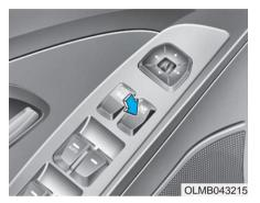
The driver can disable the power window switches on the passengers' doors by pressing the power window lock switch.
