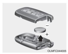
Battery Type: CR2032 To replace the battery:
