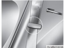
Routing the seat belt webbing through the rear seat belt guides will prevent the belts from being trapped behind or under the seats when the rear seats are folded down.
