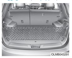
To keep items from shifting in the cargo area, use the luggage net. Make sure the luggage net is securely attached to the holders in the cargo area.
