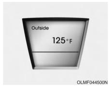
This mode indicates the current outside air temperatures by 1°F (1°C).
