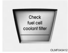
This warning message illuminates if the fuel cell coolant filter needs to be inspected or replaced. Have the vehicle inspected by an authorized HYUNDAI Tucson Fuel Cell dealer.
