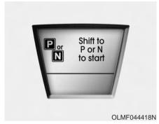
This warning message illuminates if you try to start the vehicle with the shift lever not in the P (Park) or N (Neutral) position.
